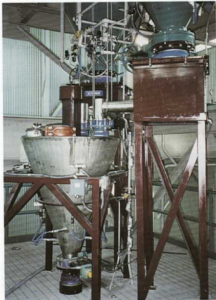
A screw feeder delivers compound ingredients from a receiving bin into a weigh hopper, which discharges into the mixer.
